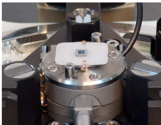
Fig. 10-7. Installing the sample on the scanner without sensors
