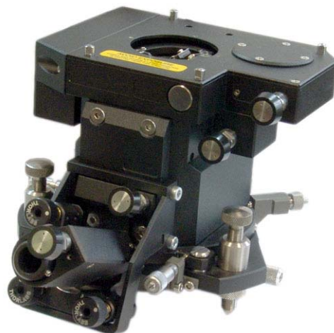
Fig. 2-17. Side illumination module installed on the measuring head
