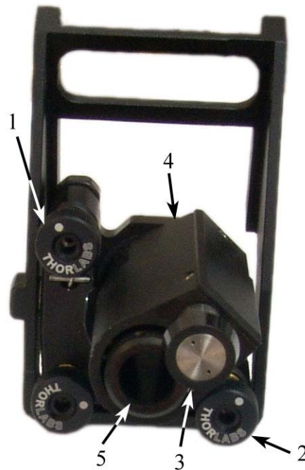
Fig. 2-16. Side illumination module 1, 2 – screws for X and Y movements of the laser spot; 3 – screw for fine focusing of the laser beam; 4 – positioning device; 5 – entrance aperture
