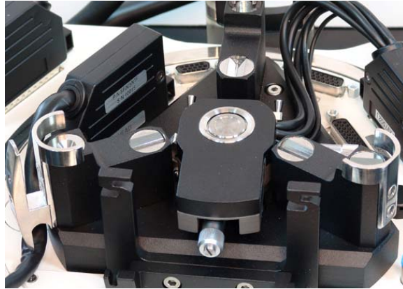
Fig. 2-5. Scanner with movement sensors mounted on the positioning device
