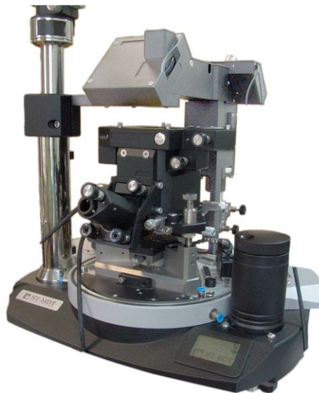
Fig. 10-21. Measuring head installed into the base unit (here the measuring head is equipped with the side illumination module)
