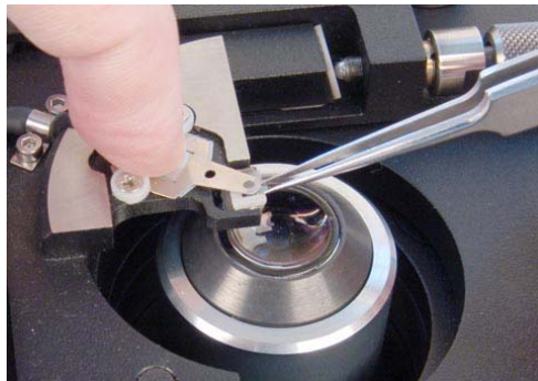
Fig. 10-18. Installing the probe
