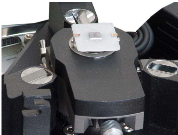
Fig. 10-4. Loading the sample into the scanner with sensors
