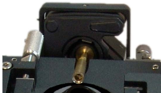
Fig. 10-14. Focusing module installed on the measuring head
