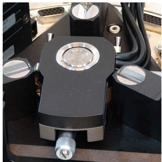
Fig. 8-7. Scanner installed in the positioning device
