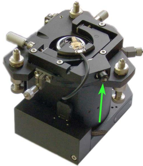
Fig. 10-15. AFM probe holder installed. Arrow indicates handle of the clamp (here the measuring head is shown without the side illumination module)
