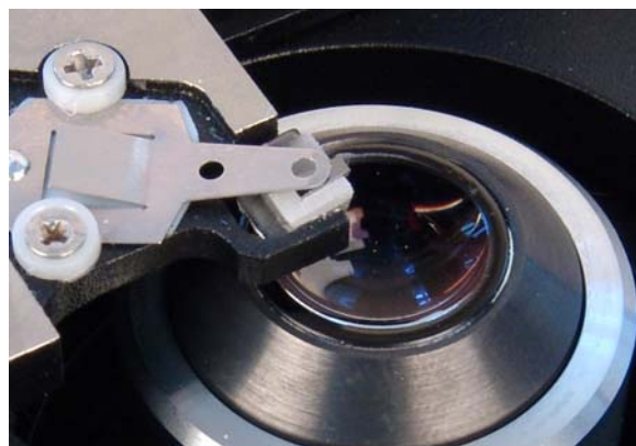
Fig. 10-19. Probe installed into the holder
